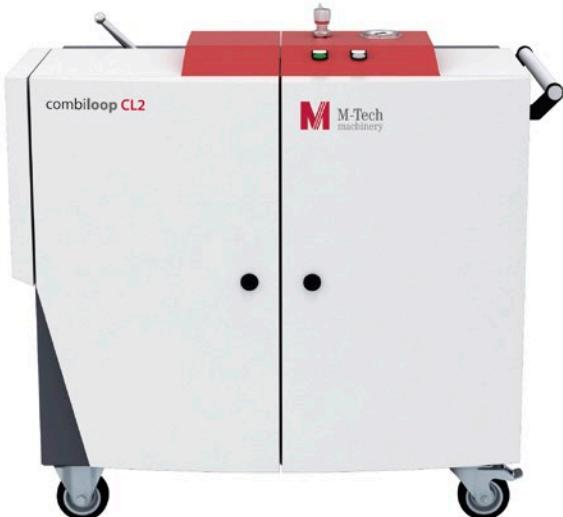
Mobile, compact high-pressure unit with 3-chamber tank system for continuous use of high pressure at machine tools. Well suited for all materials, even for materials producing fine chips like brass and aluminium. Protected function principle of preseparation of dirt in a 3-chamber tank system.
